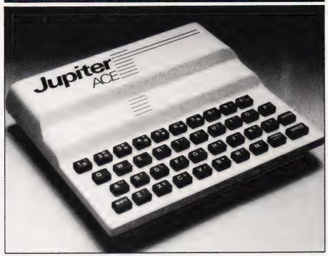
ne Jupiter Ace has only the most basic of floating point words defined in ROM. However, with a little effort, a fairly acceptable package of floating point words may be defined. Indeed, this process is started by the inclusion of floating point stack manipulation words and square root and trigonometric functions in the Jupiter Ace manual.
